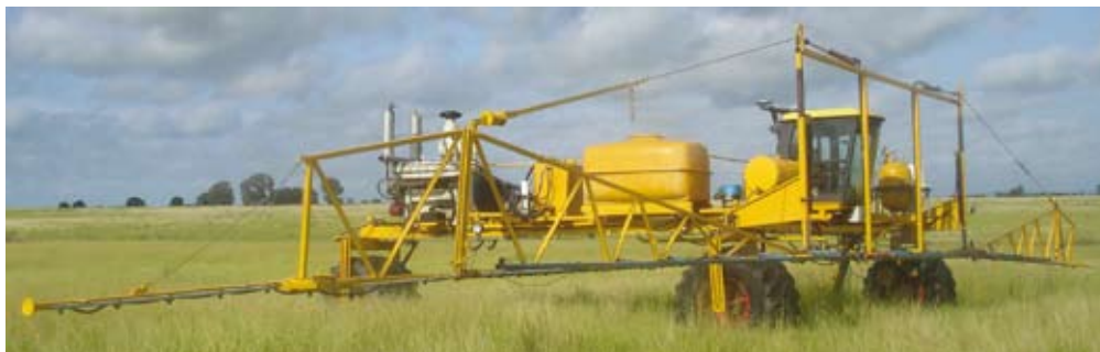
A 111 foot (34 metre) broadacre chemical sprayer designed and manufactured by Trevilyan Research. The sprayer was developed with help from the R&D Tax Concession .
