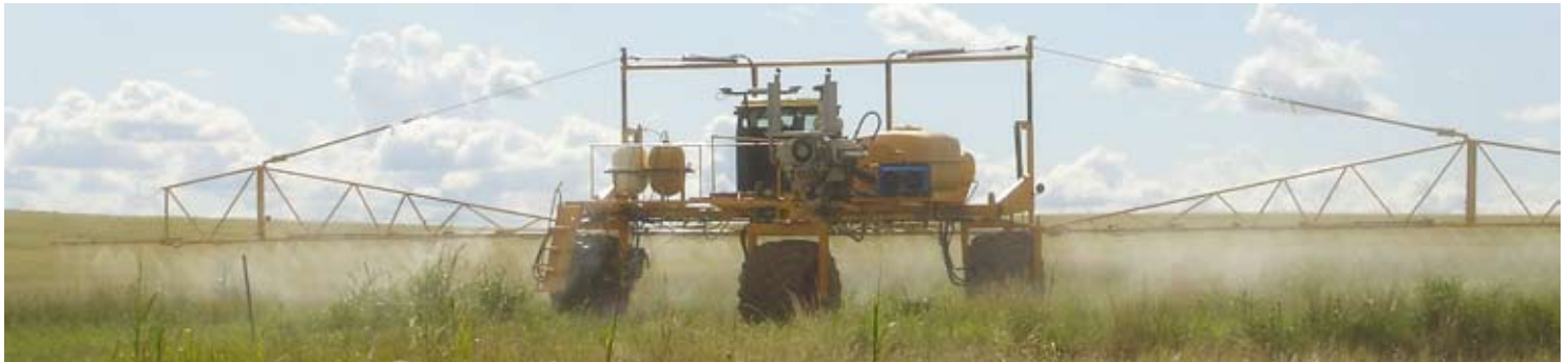
A 111 foot (34 metre) broadacre chemical sprayer designed and manufactured by Trevilyan Research. The sprayer was developed with help from the R&D Tax Concession .
